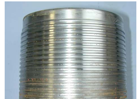
Fig. 6: External thread after 1000 h
