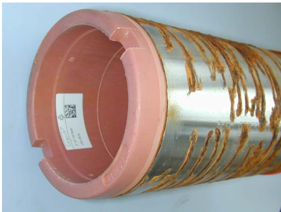
Fig. 4: Sample after 1000 h NSS-Test
