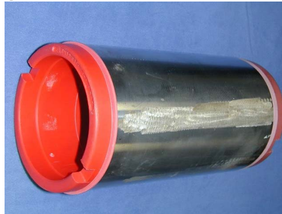
Fig. 2: Sample with assembled protectors
