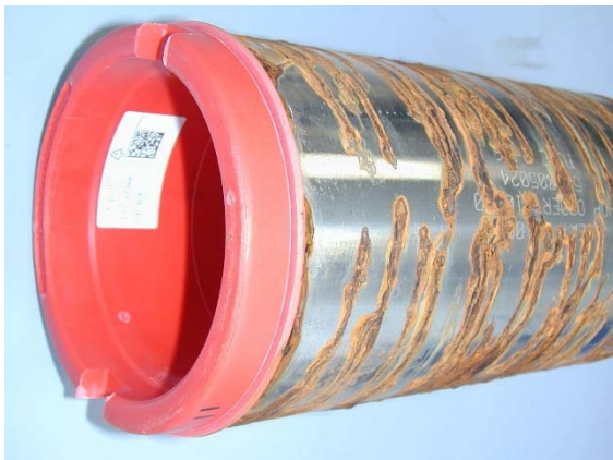
Fig. 4: Sample after 1000 h NSS-Test
