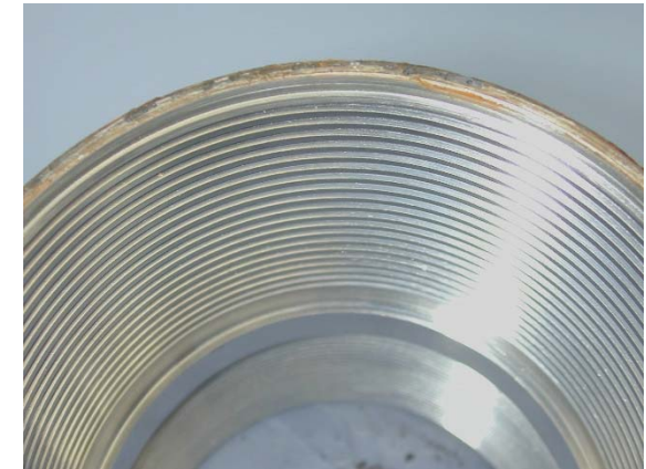
Fig. 6: Internal thread after 1000 h
