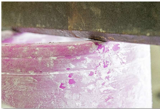
Protector after -46°C test
