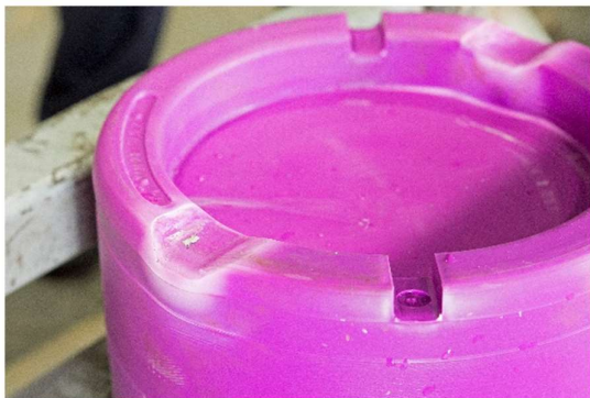
Protector after +66°C test
