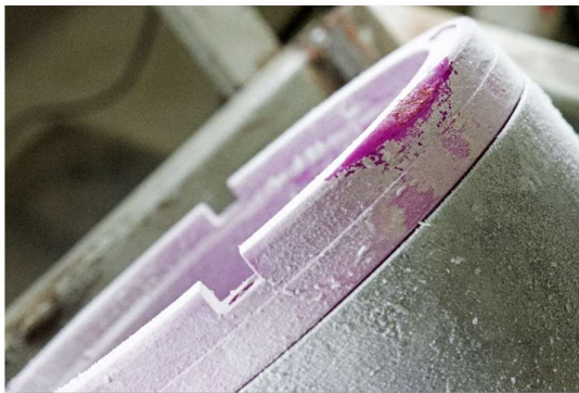
Protector after -46°C test
