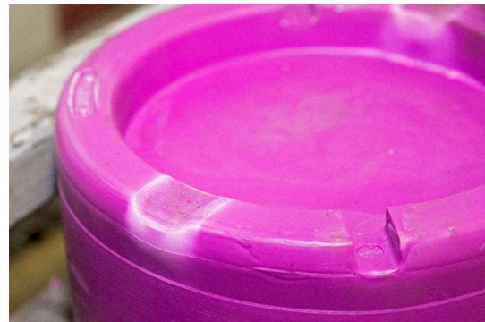
Protector after +21°C test
