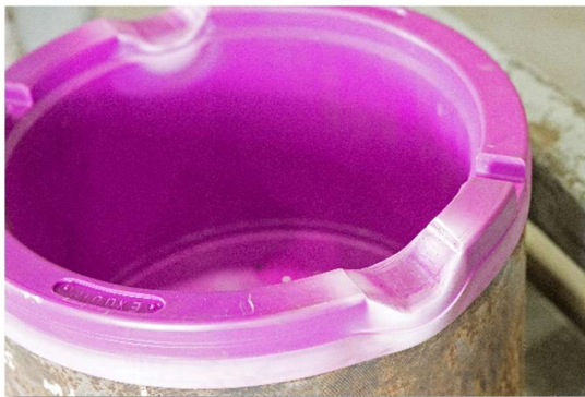
Protector after +66°C test
