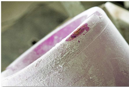
Protector after -46°C test
