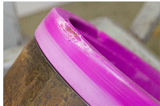
Protector after +21°C test
