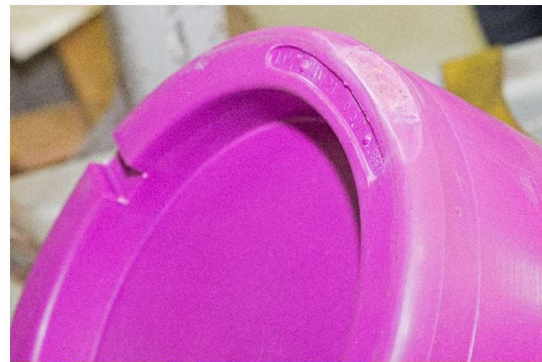
Protector after +21°C test
