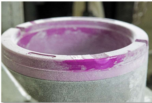
Protector after -46°C test
