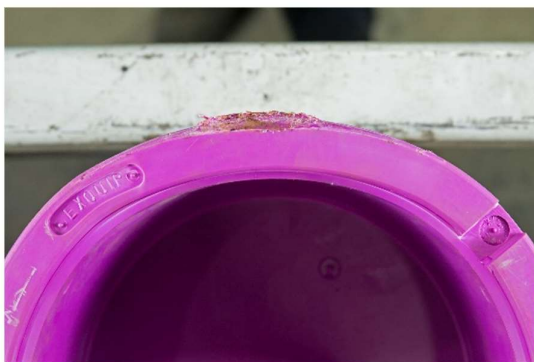
Protector after +66°C test
