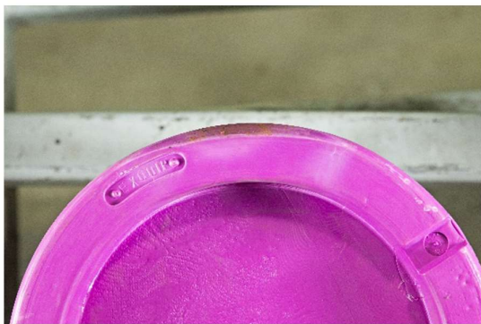
Protector after +66°C test
