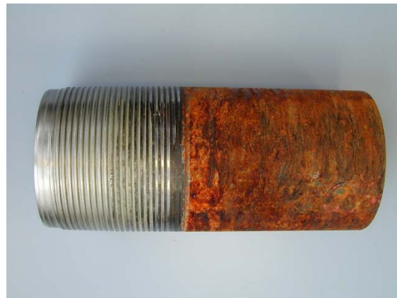
Fig. 4: Overview after 1000 h NSS-Test
