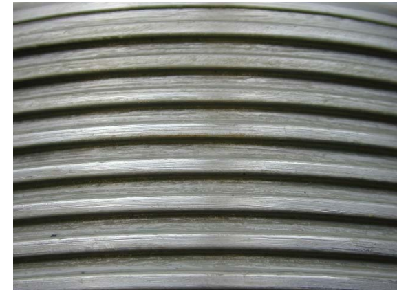
Fig. 6: External thread after NSS-Test in detail
