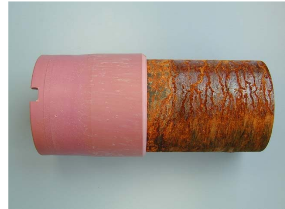
Fig. 3: Sample after 1000 h NSS-Test
