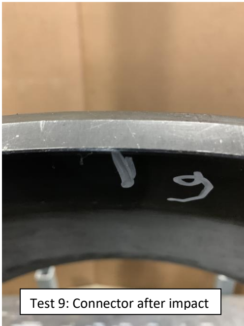
Test 9: Protector after impact
