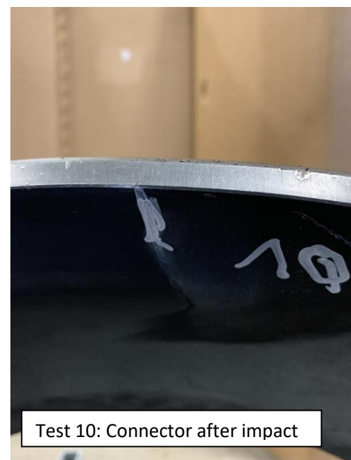
Test 10: Protector after impact
