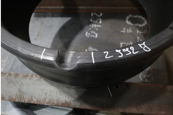
Protector (1) after testing – impact energy 2992 J
