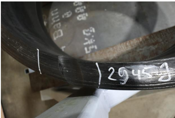
Protector (4) after testing with 2945 J
