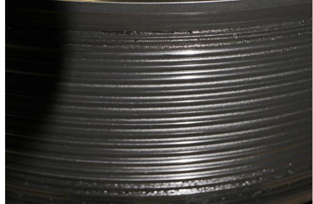
Connector threads after testing with 2992 J Protector (1)
