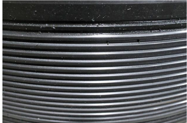
Connector threads after testing with 2992 J Protector (3)
