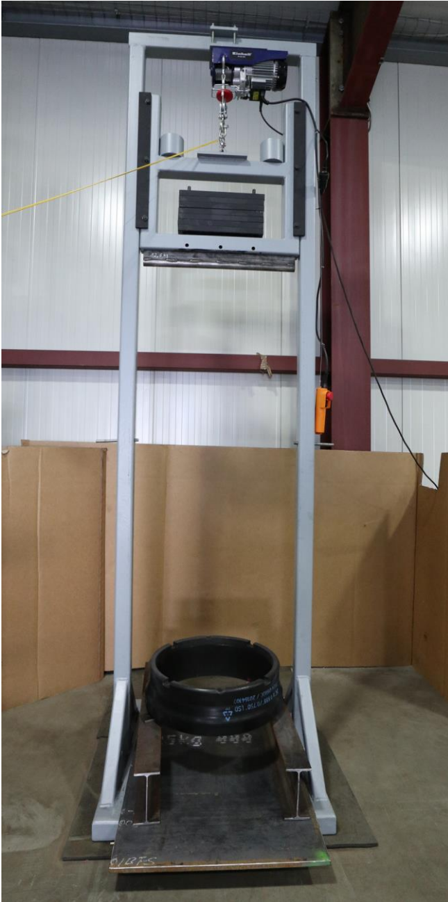
Testing device with installed protector (1) and maximum height
