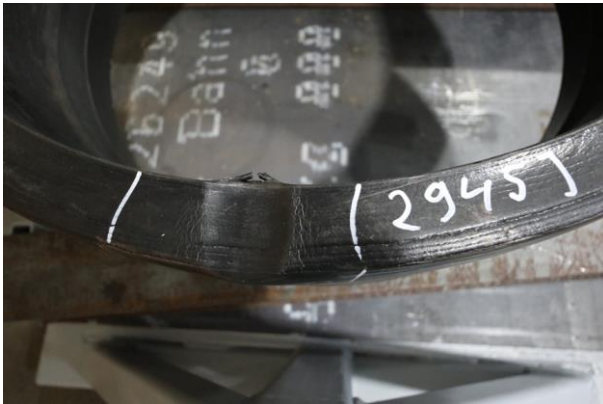
Protector (2) after testing with 2945 J
