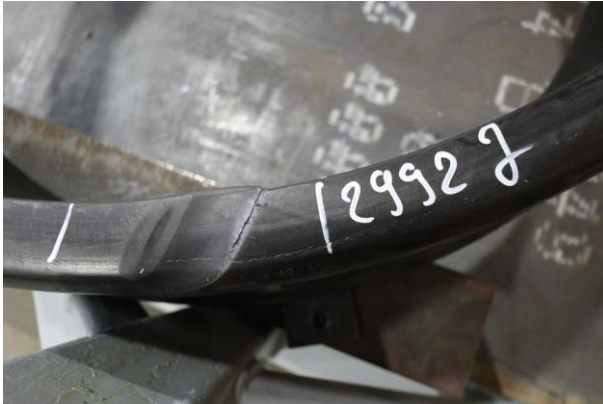
Protector (3) after testing – impact energy 2992 J
