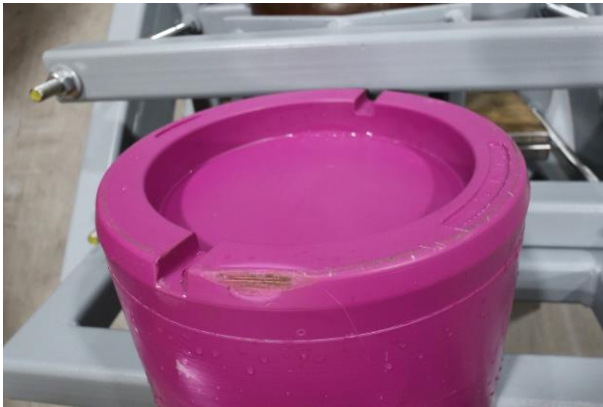
Protector (1) after testing
