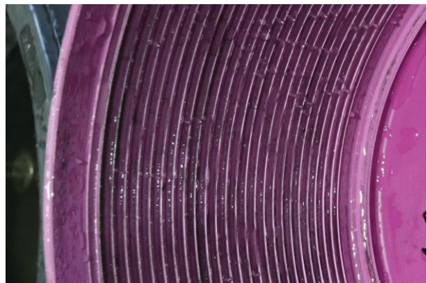
Threads of the protector after testing (1)
