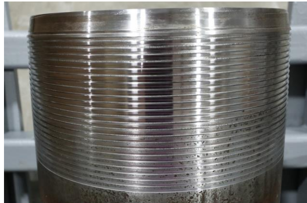
Connector threads after testing Protector (1)
